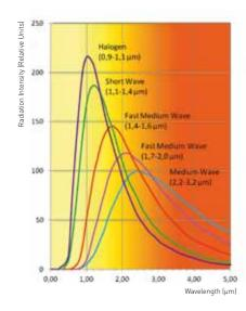
The picture on the left shows all the radiation intensity curves for halogen, short wave, medium and fast medium wave emitters.
